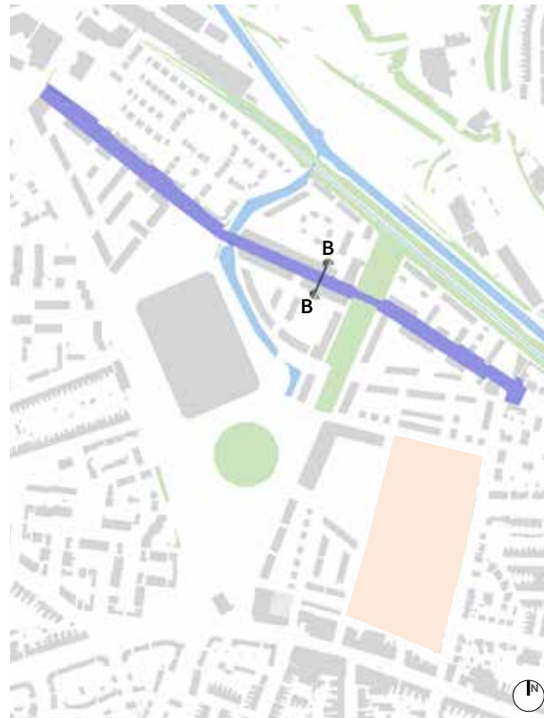
Fig. 5.25 - Cranford Street widened to accommodate the cycle route on its southern side, overlaid on masterplan
